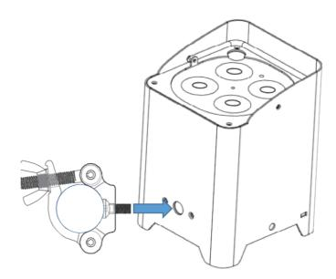
When install the fixture to crossbar or truss, always use an extra safety cord (not supplied with the fixture). Users also need to make sure the crossbar is stable or not moving, and can support a weight of 38 kg (fixture net weight 3.8kg).
