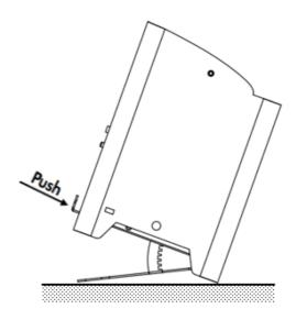
Make sure that the fixture is always placed on even and strong enough surface, and keep it 0.5m away from projection objects.
