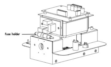
In case fuse is blown, you need to replace it. Unplug the fixture from power, remove the 4 screw from the housing to find the fuse holder. Open the fuse holder by turning it anticlockwise; remove the blown fuse from the holder and replace it with the exact same type and rating one. Close the fuse holder by turning it clockwise to tighten it. Screw back the base to the housing.
