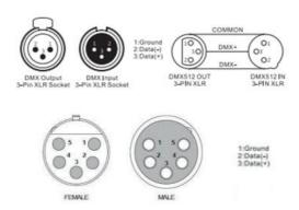
For installations where the DMX cable has to run a long distance or is in an electrically noisy environment, such as in a discotheque, it is recommended to use a DMX terminator. This helps in preventing corruption of the digital control signal by electrical noise. The DMX terminator is simply an XLR plug with a 120  $\Omega$  resistor connected between pins 2 and 3, which is then plugged into the output XLR socket of the last fixture in the chain. Please see illustrations below.
