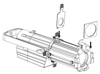
INSERT GOBO HOLDER AND GEL FRAME HOLDER INTO THE GAP SHOWED AT ABOVE PICTURE
