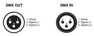
If you are using controllers with this occupation, you can connect the DMX-output of the controller directly with the DMX-input of the first fixture in the DMX-chain. If you wish to connect DMX-controllers with other XLR-outputs, you need to use adapter-cables.
