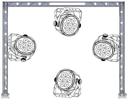
The LEDPAR720TW is fully operational in two different mounting positions, hanging upside-down from a ceiling or set on a flat level surface. To avoid internal damage to the unit, never mount the unit on its side as illustrated above. Be sure this fxture is kept at least 0.5m away from any flammable materials (decoration etc.). And you'd better use and install the supplied safety cable as a safety measure to prevent accidental damage and/or injury in the event the clamp fails (see next page).
