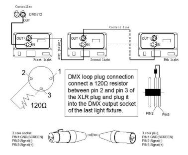
1. In order to reduce signal errors and avoid signal weakening or interference during transmission, a  $120\Omega$  resistance loop can be inserted between the 2 cores and the 3 cores of the DMX output terminal of the last machine.
