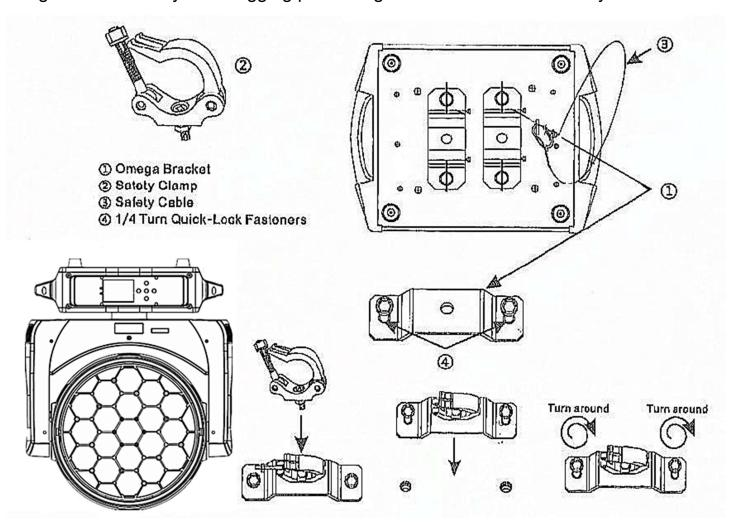
Regardless of the rigging option you choose for our fixture, always be sure to secure your fixture with a safety cable. The fixture provides a built-in rigging point for a safety cable on the hanging bracket as illustrated above. Be sure to only use the designated rigging point for the safety cable and never secure a safety cable to a carrying handle.
