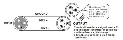
caution:Do not allow contact between the ground and the fixture's chassis ground. Grounding the ground can cause a ground loop, and your fixture may perform erratically. Test cables with an ohm meter to verify positive pole and to make sure the pins are not grounded or shorted to the shield or each other.
