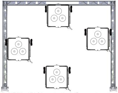
The BATMINI310LIP is fully operational in two different mounting positions, hanging upside-down from a ceiling or set on a flat level surface. To avoid internal damage to the unit, never mount the unit on its side as illustrated above. Be sure this fxture is kept at least 0.5m away from any flammable materials (decoration etc.). And you'd better use and install the supplied safety cable as a safety measure to prevent accidental damage and/or injury in the event the clamp fails (see next page).
