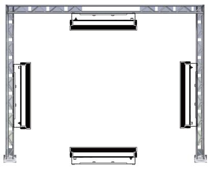
The BATBAR810LIP is fully operational in three different mounting positions, hanging upside-down from a ceiling, set on a flat level surface or mount the unit on its side. Be sure this fxture is kept at least 0.5m away from any flammable materials (decoration etc.). And you'd better use and install the supplied safety cable as a safety measure to prevent accidental damage and/or injury in the event the clamp fails (see next page).
