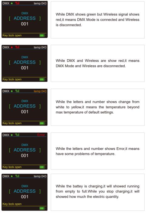
DMX-In this menu, you can connect several pieces of lights with DMX cable and control them with control console.
