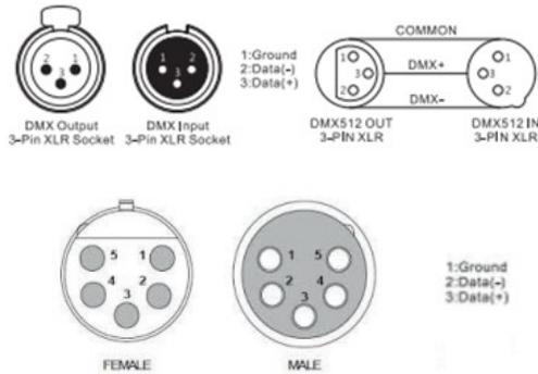
For installations where the DMX cable has to run a long distance or is in an electrically noisy environment, such as in a discotheque, it is recommended to use a DMX terminator. This helps in preventing corruption of the digital control signal by electrical noise. The DMX terminator is simply an XLR plug with a 120 Ω resistor connected between pins 2 and 3, which is then plugged into the output XLR socket of the last fixture in the chain. Please see illustrations below.
