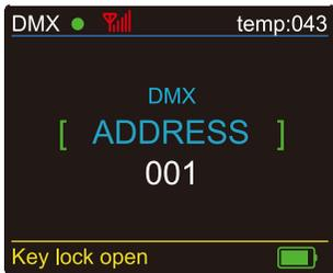
While DMX shows green but Wireless signal shows red, it means DMX Mode is connected and Wireless is disconnected.
