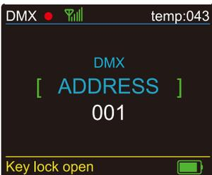
While DMX shows red but Wireless signal shows green, it means DMX Mode is disconnected and Wireless is connected.
