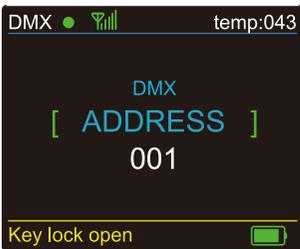
While DMX and Wireless signal are green, it means DMX Mode and Wireless are connected.
