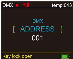
While DMX and Wireless are shown red, it means DMX Mode and Wireless are disconnected.
